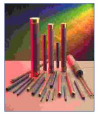
**Ferrite Rods** - Our ferrite rods are manufactured in solid, flat sided solid, hollow, fluted and fluted tube configurations, in 1mm or 2mm steps from 4mm to 20mm. Our material grades, F59 or W10, are specifically designed for tube welding applications to provide optimum performance (see our web site at <a href="https://www.mmggb.com">www.mmggb.com</a> for material properties.)
