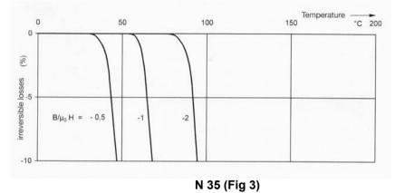
As previously stated, to achieve the minimum effect from temperature changes in a magnetic circuit, it is necessary to establish as accurately as possible, the working point of the magnet to be used. A simple curve showing the irreversible losses for N35 grade NdFeB at various working points is shown in Fig. 3. The working point (B/ $\mu_0$ -H) for high coercive materials can be calculated by using the following method for a single discrete magnet with no iron circuit.
